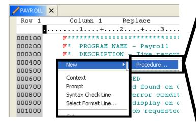
Procedure wizard generates prototype and body stub
